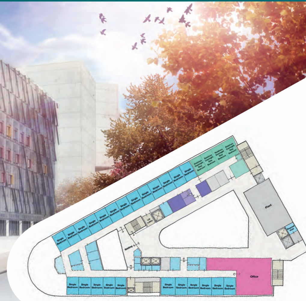
Draft plan for a floor of inpatient beds. Every inpatient will have their own single room
