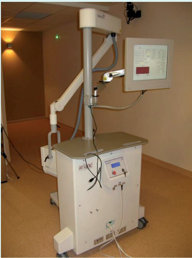
Figure 6. The Papillon 50™ system installed in Centre Antoine Lacassagne. The micronode is stored in the parking stand.
