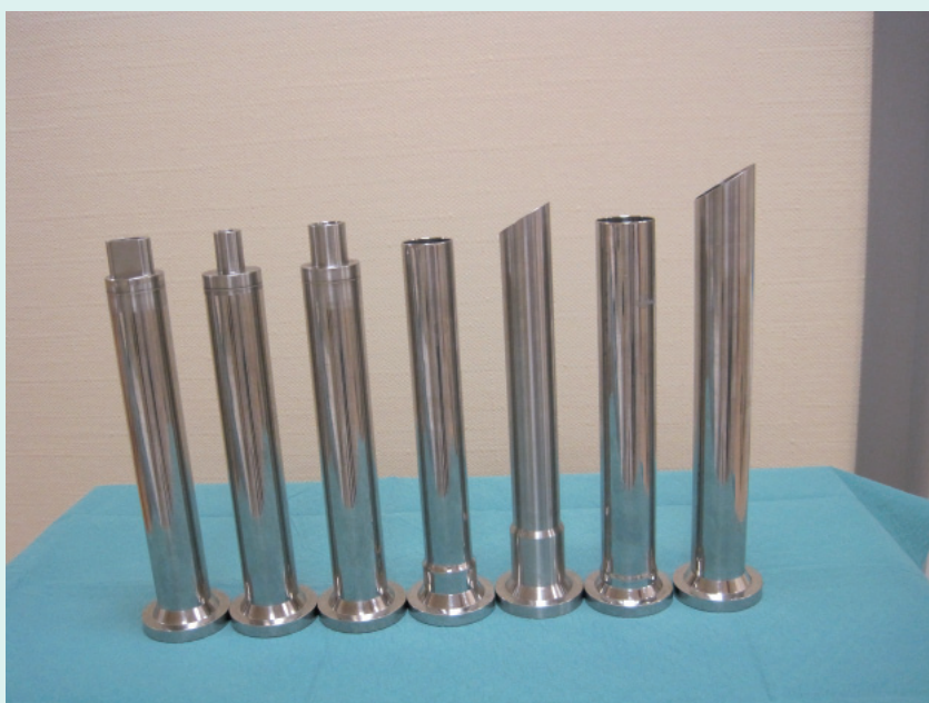
Figure 8. Applicators used with the Papillon 50™ from left to right: eyelid applicator (1 cm), skin applicator (1, 1.5 cm), rectal straight (2.5 cm), rectal oblique (2.5 cm), rectal straight (3 cm) and rectal oblique (3 cm).
