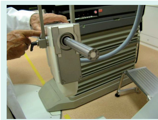
Figure 9. Extremity of the micronode showing the channel for camera, cold light and cooling.
